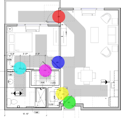
A5 UNIT PLAN AL-B2.5 1/4" = 1'-0" 122 OSF - 2 UNITS TOTAL
