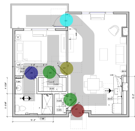
A4 UNIT PLAN AL-B2.1 1/4" = 1'-0" 700 GSF - 3 UNITS TOTAL
