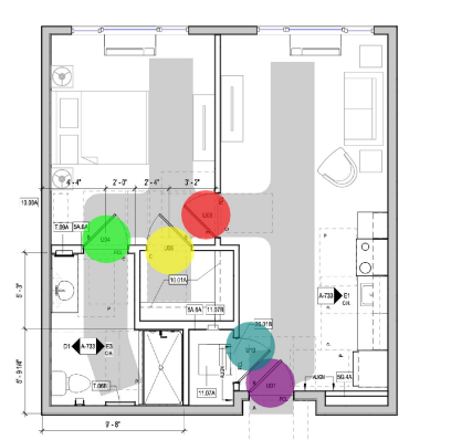
A4 UNIT PLAN IL-B1.0 14'4" x 11'0" 624 GSF - 5 UNITS TOTAL
