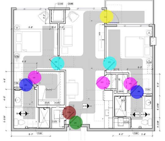
A3 UNIT PLAN AL-D2.0 144" x 110" 1008 GSF - 8 UNITS TOTAL
