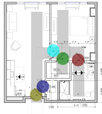
A4 UNIT PLAN AL-B1.1 1/4" = 1'-0" 624 GSF - 4 UNITS TOTAL
