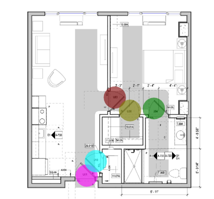
A3 UNIT PLAN IL-B1.1 14'4" x 11'0" 624 GSF - 5 UNITS TOTAL
